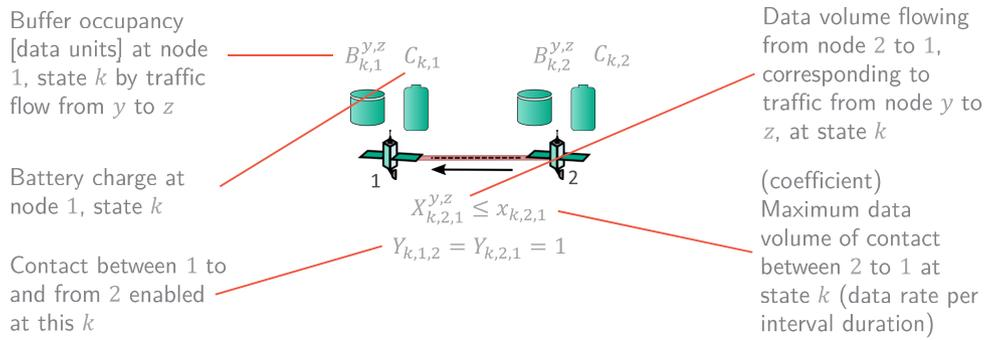
FIGURE 4 Traffic flow, buffer occupancy, battery charge and binary decision variables of the model.
