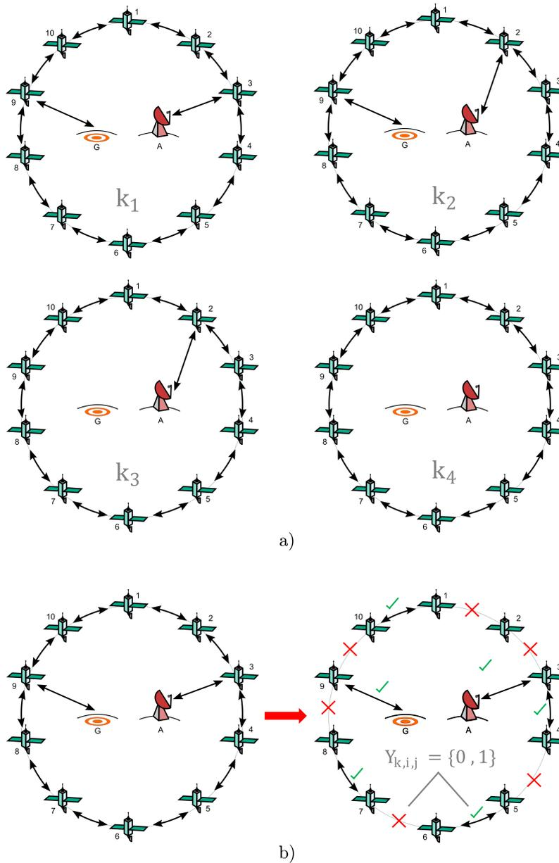
**FIGURE 3** Time-evolving topology model based on discrete time episodes  $k_1, k_2, k_3$  and  $k_4$  in a). This model facilitates the scheduling of contacts on each of this episodes via  $Y_{k,i,k}$  boolean variables as shown in b)<sup>6</sup>
