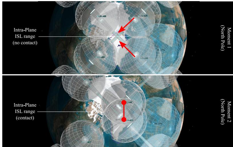
**FIGURE 2** Intra-plane ISL is achieved via wide beam-width antennas in the pole areas, when satellites are in range (i.e., moment 2).
