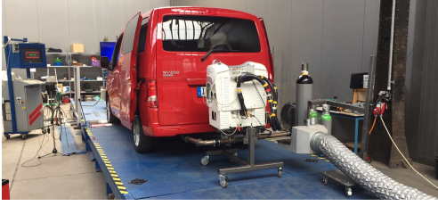
Fig. 5. Nissan NV200 Evalia on a dynamometer
