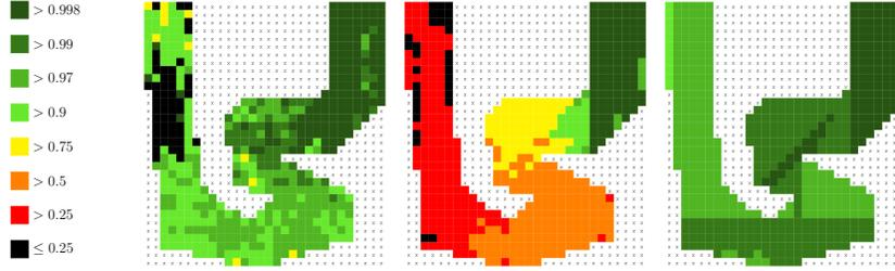
**Fig. 3.** Goal probability of NN oracle on the Barto-big benchmark trained and executed with 20% noise vs. stress-test executed with 50% noise using the same NN (middle) vs. optimal policies obtained by probabilistic model checking with 50% noise (right).
