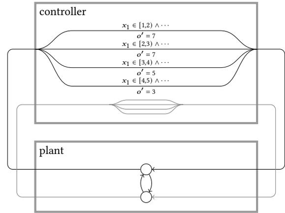
Figure 3: Structure of a hybrid automaton for a cyber-physical system with a discrete controller
