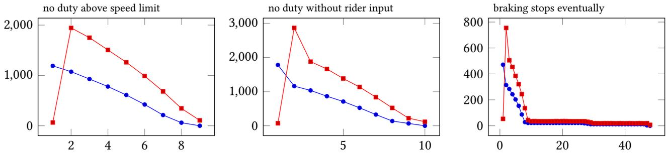
Figure 5: Execution time (—■—, in milliseconds, y axis) and number of chunks produced (—●—, y axis) per cycle (x axis). The time in the first cycle is always low because the initial state is represented by a single box; the number of boxes generated influences the number of intersections needed in the *next* cycle.
